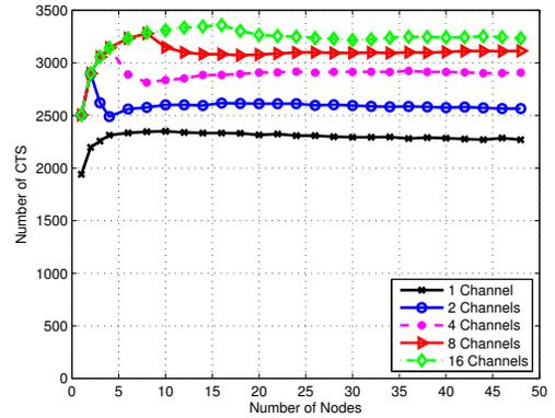
Fig. 7: Number of CTS messages for different  $c_{max}$  vs. number of nodes.
