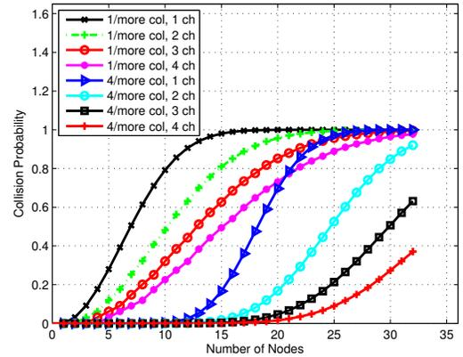
Fig. 3: Probability for different number of collisions in sub-channelized DCF vs. number of nodes.
