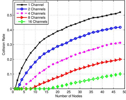
Fig. 8: RTS collision rate for different  $c_{max}$  vs. number of nodes.
