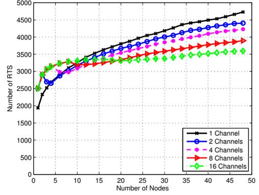
Fig. 6: Number of RTS messages for different  $c_{max}$  vs. number of nodes.
