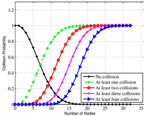
Fig. 2: Probability for different number of collisions vs. number of nodes.
