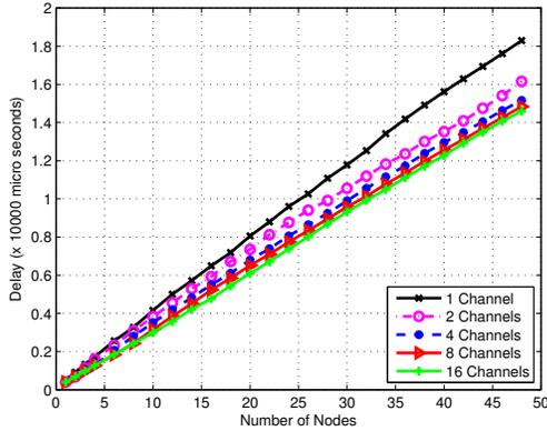
Fig. 9: Average packet delay for different  $c_{max}$  vs. number of nodes.
