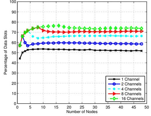
Fig. 10: Percentage of time the channel is used for carrying payload data vs. number of nodes for different  $c_{max}$ .
