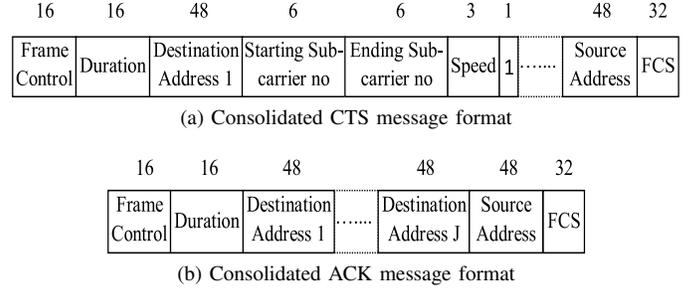
Fig. 5: Enhanced IEEE 802.11 CTS/ACK messages for dynamic OFDMA signalling.
